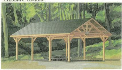
Note: Finish Roof (shingles/metal) supplied by owner. All timbers to be cut on site. Precutting is available at an additional charge. Custom sizes are available. The image below shows the standard frame without the optional 2x6 Tongue & Groove. Shelters 28' wide and less are Eastern White Pine. Shelters over 28' wide are Southern Yellow Pine.
